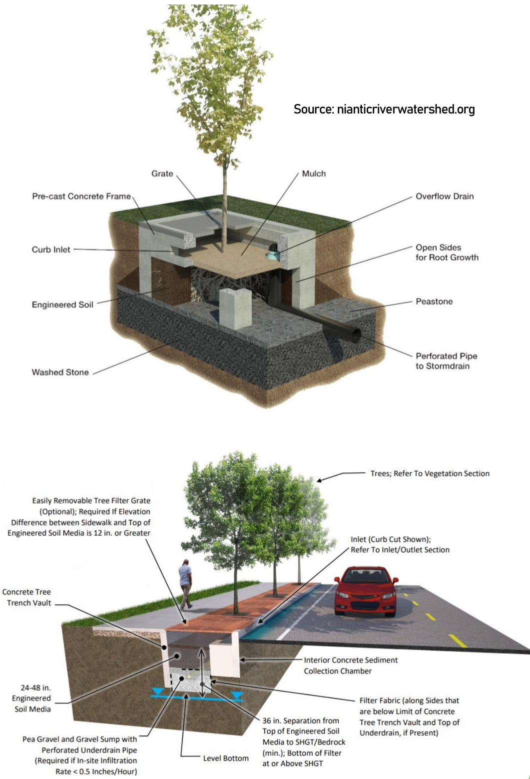
Figure 13-19. Tree Filter with Underdrain Schematic
