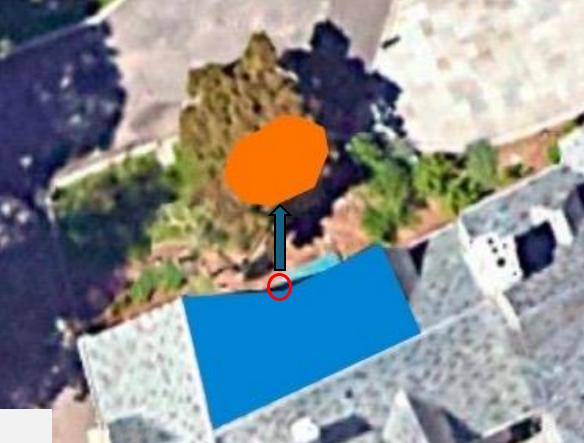
Key: Drainage area Rain garden O = drain T = water flow
