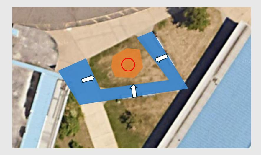
Key: Drainage area Rain garden Q = drain 1 = curb cuts
