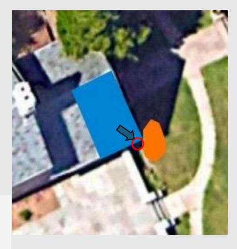
Key: Drainage area Rain garden O = drain T = water flow
